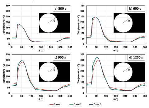
Figure 3: Outer wall temperature profiles at 300 s (a), 600 s (b), 900 s (c) and 1200 s (d) as a function of the angular coordinate  $\theta$ , defined in Figure 1.
