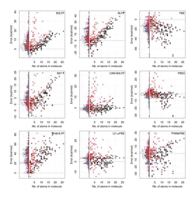
FIG. 6. Distribution of the errors for AE as a function of the number of atoms in the molecules of the G3/99 set for nine DFAs. The data points are coded for CHON-type molecules (gray squares and histogram) and the other ones (red circles and histogram). The histograms corresponding to the partial and whole datasets are displayed in the left panel of each graph. The histogram for the whole dataset is traced with blue lines.
