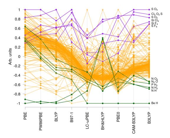
FIG. 8. Parallel plot of the IAE errors in the G3/99 dataset. All error sets have been linearly rescaled to a common [-1, 1] range. Lines join identical molecules in each set. The DFAs have been ordered to display similarity in outliers patterns. The labels on the right show selected outliers for B3LYP.
