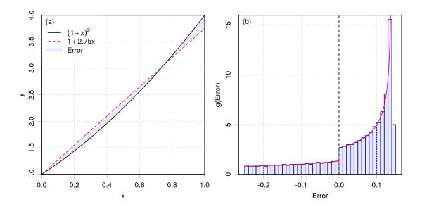
FIG. 1. Model error distribution for the least-squares approximation of the curve  $y = (1 + x)^2$  by the linear model  $\tilde{y} = 1 + 2.75x$ . (a) the curves and errors on  $x \in [0, 1]$ ; (b) the probability density of errors g(Error) (red curve) and a histogram for a uniform sample of x.
