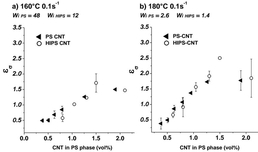
Figure 14 : Evolution of the Hencky strain value when the composites conductivity reaches  $10^{-6}$  S/cm as a function of the filler volume fraction for the two types of matrix for specimen under extensional rate fixed at  $0.1 \text{ s}^{-1}$  at 160°C a) and at 180°C b)
