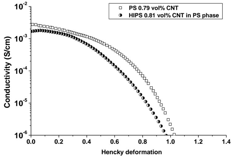
Figure 9 : Conductivity evolution under extensional deformation at 180°C for an extensional rate of 0.01 s<sup>-1</sup>
