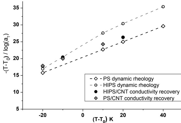
Figure 11 : WLF plot for the  $a_T$  shift factor from the build of the master curve of the pure matrices and from the build of the master curve of conductivity recovery. The reference temperature ( $T_0$ ) is 180°C
