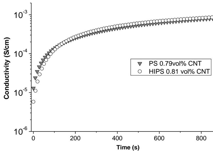
Figure 12 : Conductivity recovery under quiescent condition at 170°C of PS filled 0.79 vol% CNT and HIPS filled with 0.82 vol% CNT after a Hencky deformation of 1 at 170°C and 0.01 s<sup>-1</sup>
