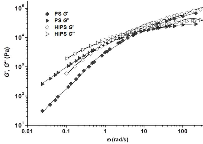
Figure 1 : Master curve of PS (filled symbols) and HIPS (open symbols) matrices built for a reference temperature of 200°C. Symbols: Experimental data  $G'$  and  $G''$ , Solid lines: Discrete Maxwell model.
