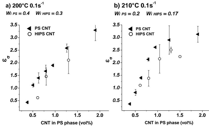
Figure 15 Evolution of the Hencky strain value when the composites conductivity reaches  $10^{-6}$  S/cm as a function of the filler volume fraction for the two types of matrix for specimen under extensional rate fixed at  $0.1 \text{ s}^{-1}$  at 200°C a) and at 210°C b)
