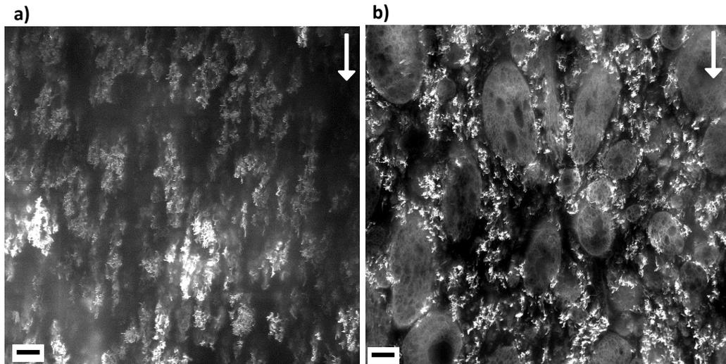
Figure 10 : SEM micrographs of the two composites after a Hencky deformation of 1 at 160°C and 0.01 s<sup>-1</sup> a) PS filled with 0.79 vol% CNT, b) HIPS filled with 0.82 vol% CNT in the PS phase and the conductivity is around 8.10<sup>-5</sup> S/cm for the two specimens. The scale bar is 2μm.
