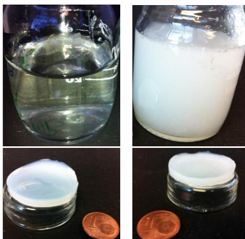
Figure 4. Reference solution (Top-left) and hydrogel (Bottom-left) of chitosan 2% ( w/w ). Solution of CHI 2% ( w/w ) filled with cellulose nanofibers 0.4% ( w/w ) (CNF/CHI suspension, Top-right) and resulting CNF/CHI composite hydrogel (Bottom-right). All samples were obtained by the aqueous route.
