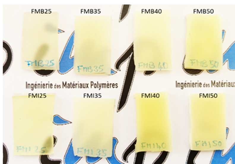
Figure 2: Visual appearance of the 2 mm thick sample sheets. First row: FMB sample series – Second row: FMI sample series. HS ratio increases from left to right
