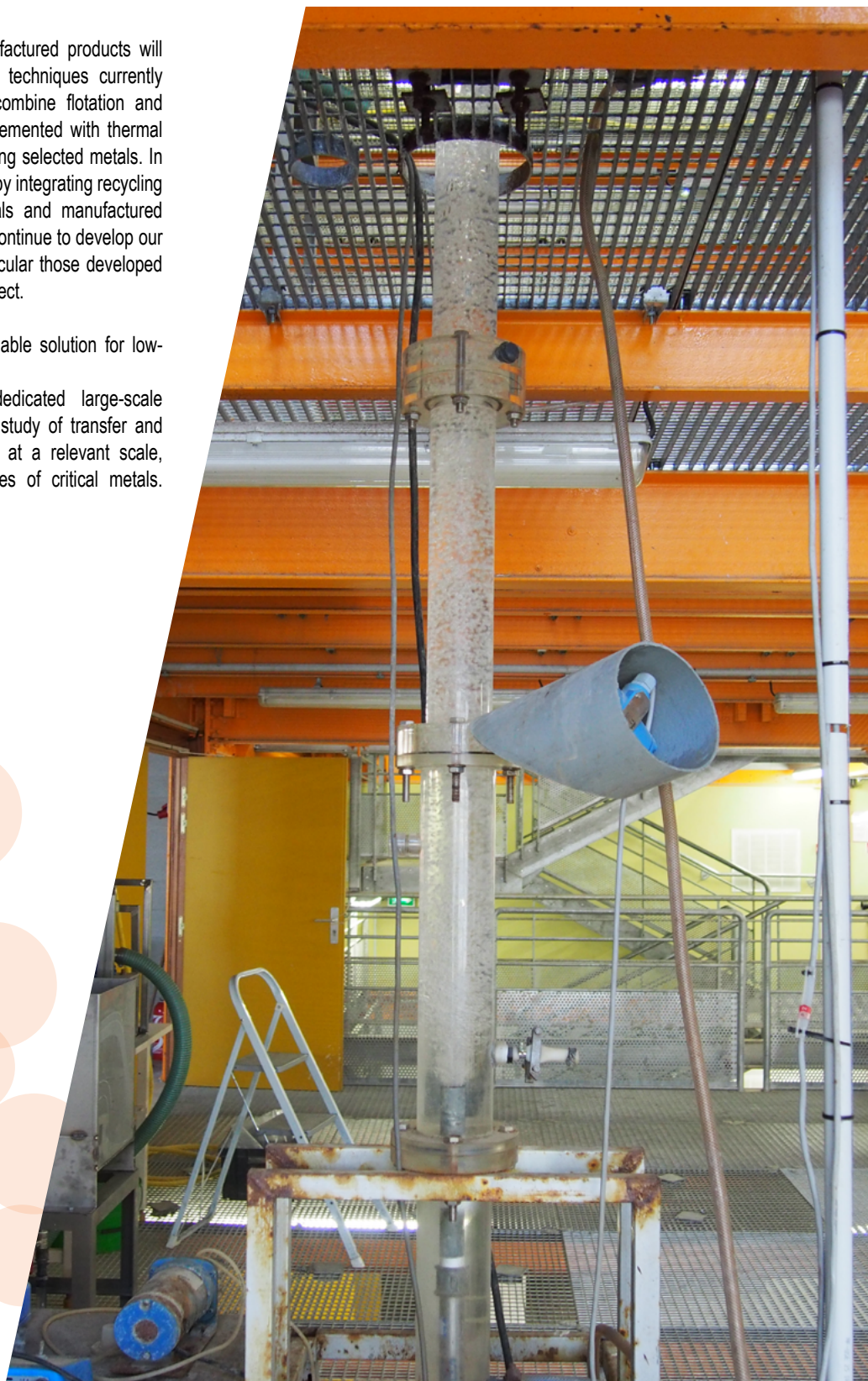
The Steval platform fore ore processing (flotation column)
