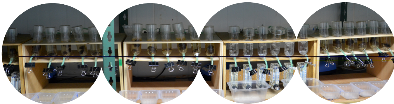
Fig. 3.5: Experimental design used to assess the effects of silver nanoparticles on the fine particulate organic matter production in Grammarus sp.
