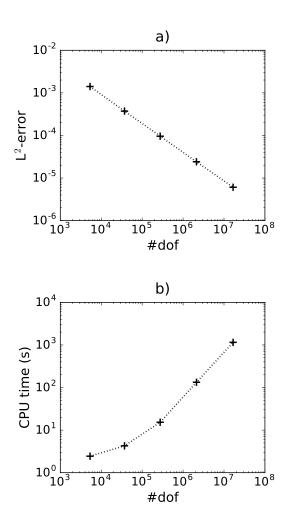
Figure 3: FSM-DG results from the first numerical example in 3D: L<sup>2</sup> error and CPU time with respect to the number of degrees of freedom. The curved shape for small number of degrees of freedom when the CPU time is lower than 10 seconds is explained by initialization steps in the code that do not depend on the size of the mesh, such as model reading and source handling, for instance.
