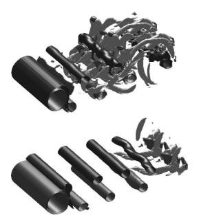
FIG. 5. Isovorticity surfaces after activation of the rotation with  $S_f = 2S_t$ . Above: t = 120, below: t = 130. Rotation starts at t = 110.
