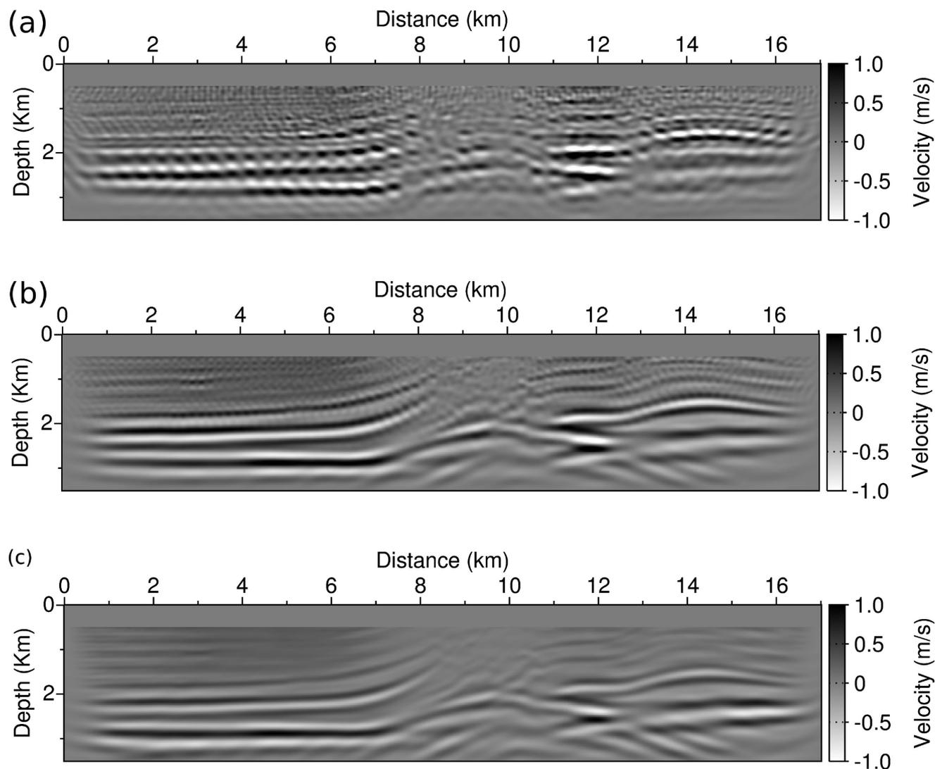
**Figure 11.** Marmousi2 case study. Effect of the compression level used for computing the Beylkin operator  $\mathcal{B}(m_0)$ . Gradient of the modified misfit function  $g(m)$  with 400, 200 and 100 m grids.
