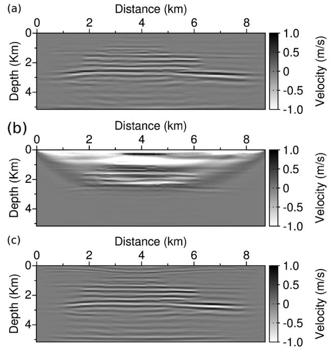
Figure 18. Model update  $\mathcal{B}(m_0)(d_{\text{cal}}(m_0) - d_{\text{obs}})$  which would be provided by the Beylkin method (a), standard FWI gradient in the initial Valhall model (b) and gradient of the modified misfit function  $g(m)$  in the initial Valhall model (c).
