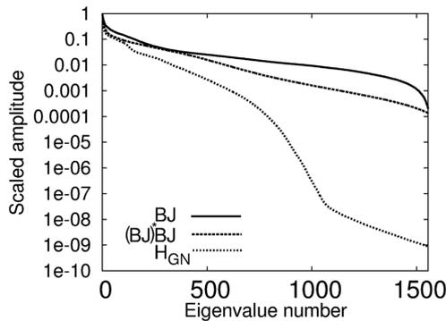
**Figure 4.** Eigenvalue distribution of the Gauss–Newton operator associated with the standard FWI misfit function  $H_{GN}(m_0)$ , the product of the Beylkin and the Born modelling operators  $\mathcal{B}(m_0)J(m_0)$ , the Gauss–Newton operator  $H_{GN}^g(m_0) = (\mathcal{B}(m_0)J(m_0))^* \mathcal{B}(m_0)J(m_0)$  associated with the modified misfit function  $g(m)$ .
