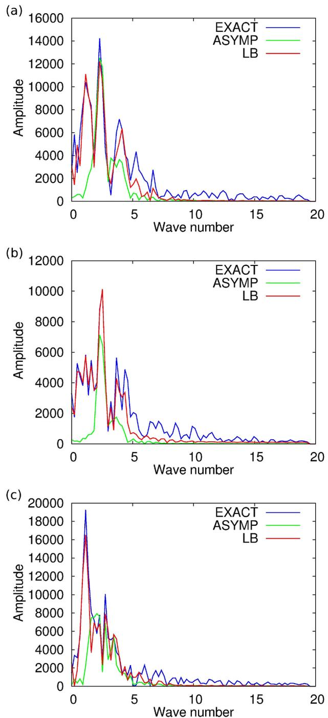
**Figure 15.** Marmousi2 case study. Wavenumber spectrum of the  $P$ -wave velocity update along vertical logs extracted at  $x = 5$  km (a),  $x = 9$  km (b) and  $x = 14$  km (c). Exact update (blue), update obtained after 10 iterations of modified FWI (green) and update obtained after 40 iterations of standard FWI (red).
