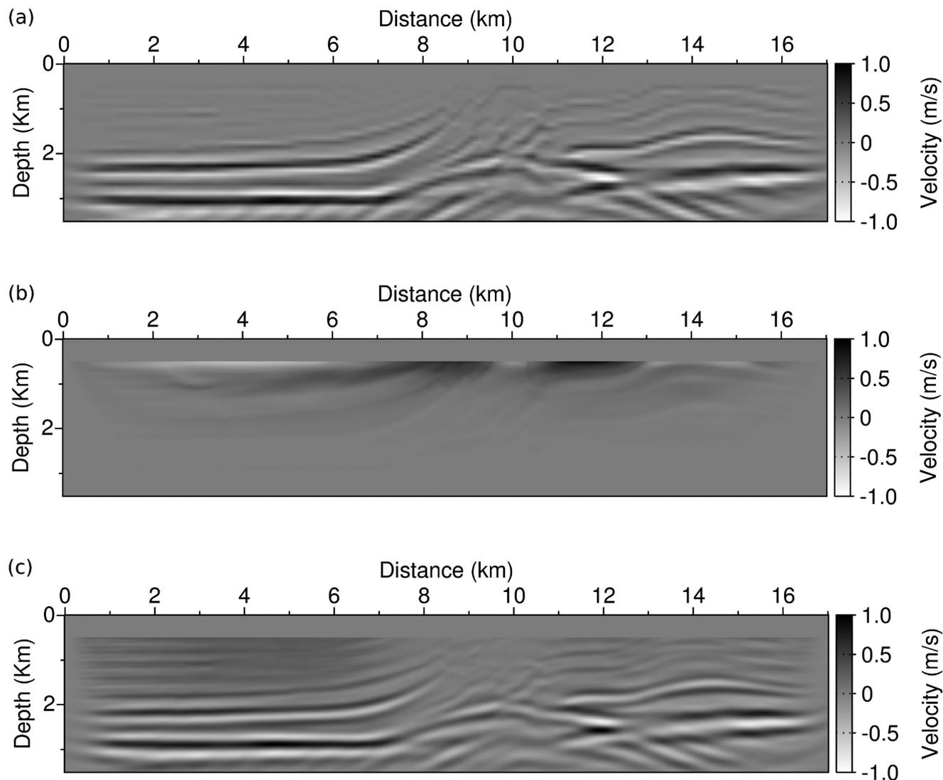
**Figure 9.** Model update  $\mathcal{B}(m_0)(d_{\text{cal}}(m_0) - d_{\text{obs}})$  which would be provided by the Beylkin method (a), standard FWI gradient in the initial Marmousi 2 model (b) and modified misfit function gradient in the initial Marmousi 2 model  $\nabla g(m_0)$  (c).
