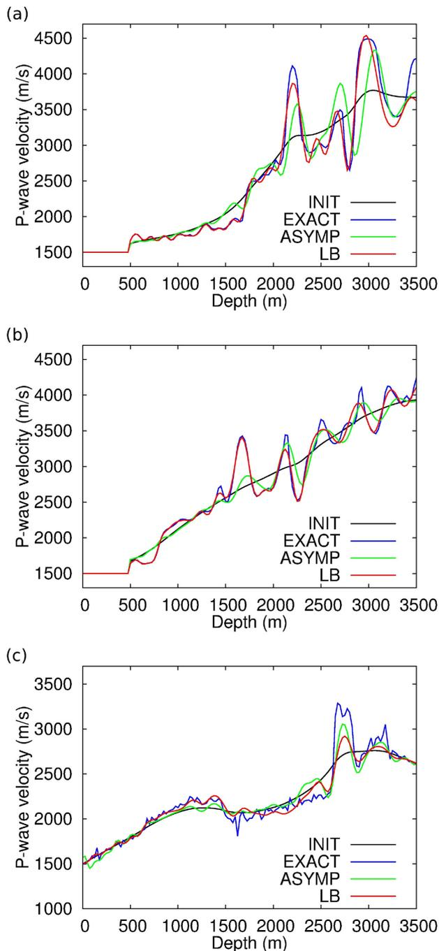
**Figure 14.** Marmousi2 case study. Vertical logs of  $P$ -wave velocity models extracted at  $x = 5$  km (a),  $x = 9$  km (b) and  $x = 14$  km (c). Exact model (red), initial model (black), reconstructed model after 10 iterations of modified FWI (green) and reconstructed model after 40 iterations of standard FWI (blue).
