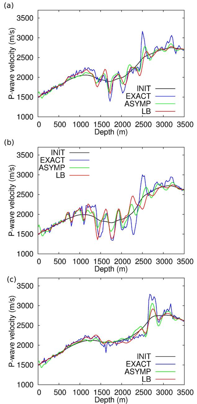
**Figure 21.** Valhall case study. Vertical logs of *P*-wave velocity models extracted at  $x = 2.1$  km (a),  $x = 4.4$  km (b) and  $x = 6.2$  km (c). Exact model (blue), initial model (black), reconstructed model after 10 iterations of modified FWI (green) and reconstructed model after 40 iterations of standard FWI (red).
