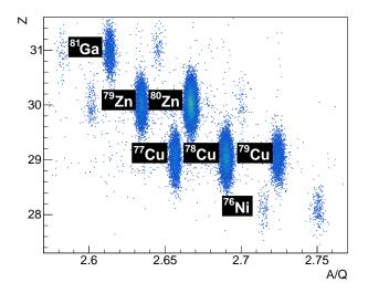
Figure 2. Particle identification of the incoming cocktail beam in coincidence with outgoing <sup>76</sup>Ni ions tagged in the ZeroDegree spectrometer and protons detected in the MINOS device.
