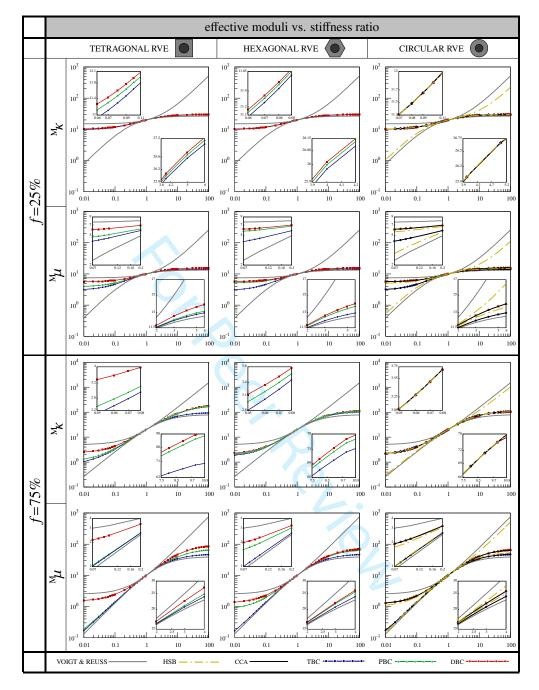
Figure 8: Overall moduli versus stiffness ratio in a logarithmic scale. Two specific volume fractions are considered that are represented in each row. A good agreement of the results is observed for the volume fraction f=25%. Increasing the volume fraction to f=75% leads to more distinguishable results. More accordance between the results is observed for the bulk modulus  $^{M}\!\kappa$  compared to the shear modulus  $^{M}\!\mu$ . The zoom boxes provide for further clarity.
