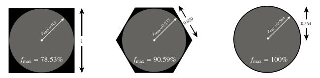
Figure 4: Maximum reachable volume fraction for each RVE. For the circular RVE, the inclusion can embed the whole RVE due its geometry.
