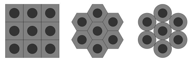
Figure 3: Packing network for each RVE. Tetragonal RVE packing (left). Hexagonal RVE packing (center) and the circular RVE packing (right). The boundaries of the tetragonal and hexagonal RVEs completely match.
