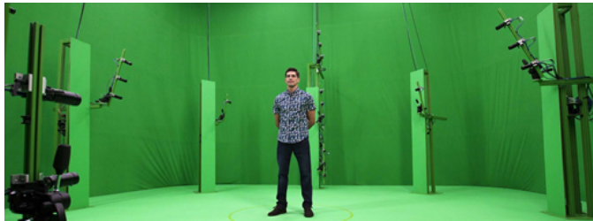
Fig. 2. Example studio for capturing dynamic point clouds.
