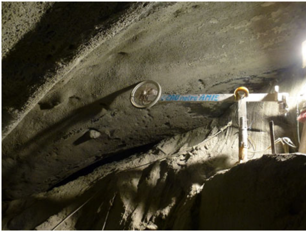
Fig. 5. Subglacial observatory with the bicycle wheel used to measure the basal motion. The articulated arm is 1.30 m long (Photograph from Luc Moreau).
