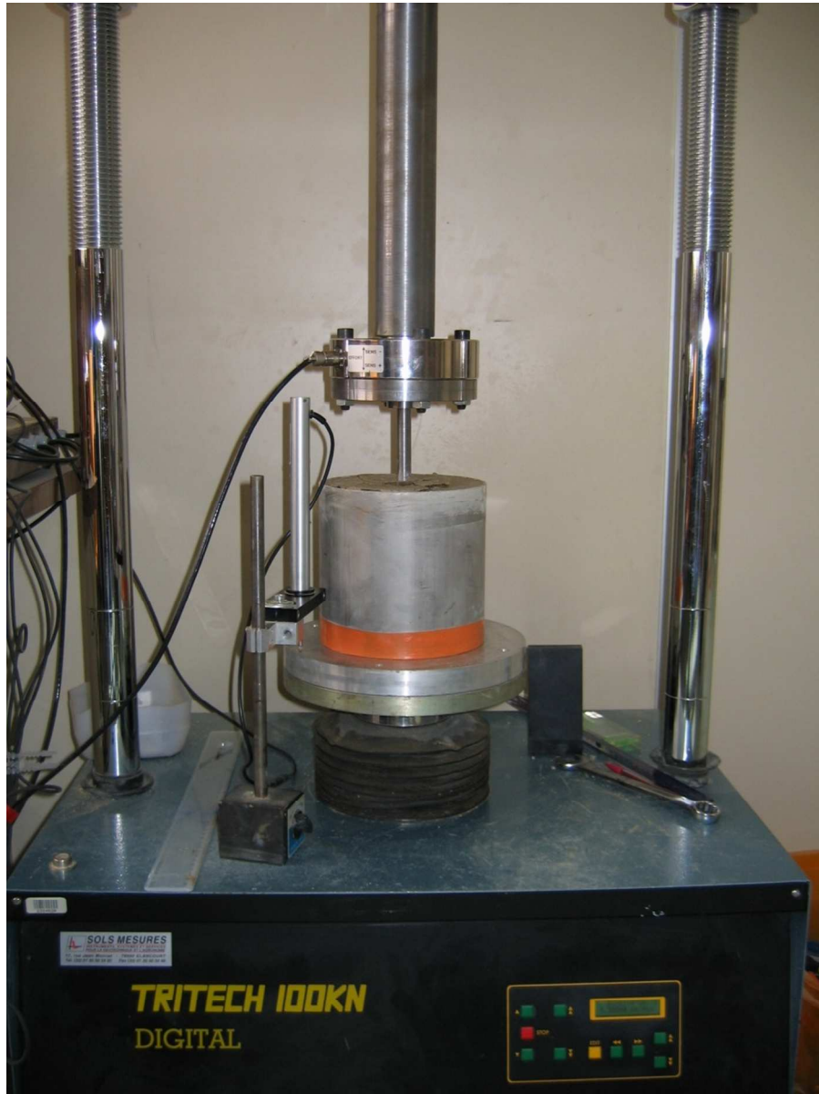
Figure 7: punching test device
