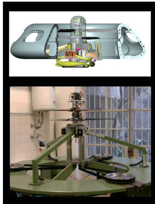
Fig.8 – Preliminary design of the RPV and tests of the propulsion system
