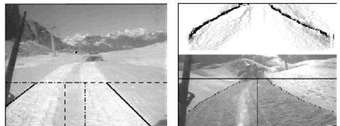
Fig. 3 – Examples of the AV results obtained with the Hough transform algorithm and with ACO (Ant Colony Organisation) algorithm. The result is the detection of the path to follow during a multivehicle raid.
