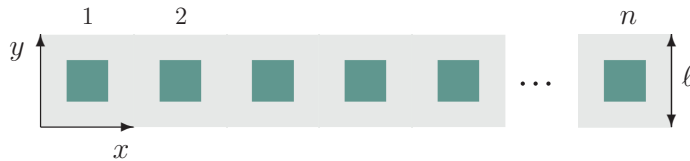
FIGURE 4. Solution domain for the direct numerical simulations consisting of an array of n inline square unit cells of length \ell .
