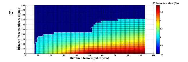
Fig. 3 Example of filtration channel charts. a) after data extrapolation and interpolation; b) after a further exclusion of bulk part. Data source: Lap1-tspp6, extracted from Fig.12 of Ref. [11]:  $T = 25\pm1^{\circ}\text{C}$ ,  $TMP = 1.1\times10^{5}$  Pa,  $Q_{v} = 0.3$  L.min<sup>-1</sup>, without US.
