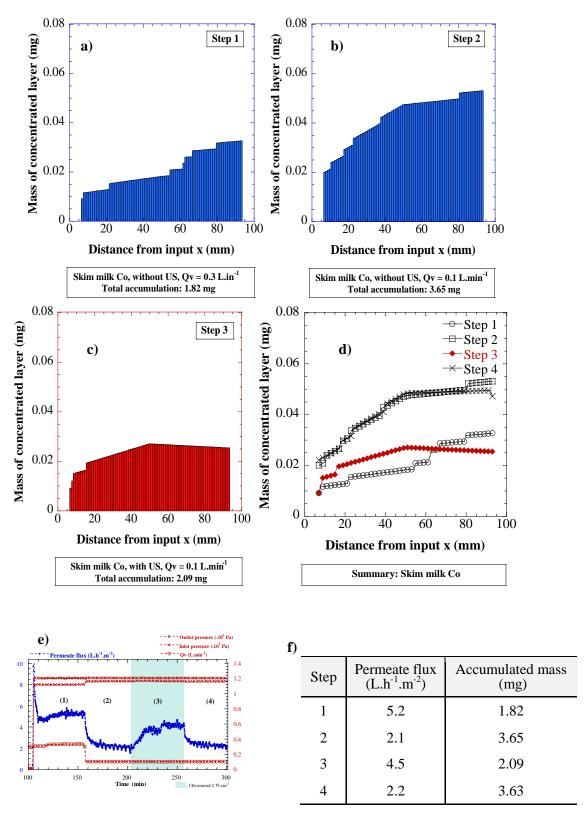
Fig. 6 Matter accumulation of concentrated layer along x axis during filtration of skim milk suspensions (feed:  $C_o$ ).  $T = 25\pm1^{\circ}C$ ,  $TMP = 1.1\times10^{5}$  Pa. US: 20 kHz, 2 W.cm<sup>-2</sup>. a-d: mass profiles; e: reminder of permeate flux  $J_v$  curve for step 1 to 4; f: table of values for each step at steady state.
