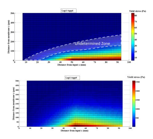
Fig. 10 Charts of yield stress during filtration of Laponite dispersions. a) Lap1-tspp6, b) Lap1-tspp0. Operating conditions: steady state,  $T = 25\pm1^{\circ}C$ ,  $TMP = 1.1\times10^{5}$  Pa,  $Q_v = 0.3$  L.min<sup>-1</sup>.
