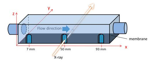
Fig. 1 Schematic view of the designed filtration cell
