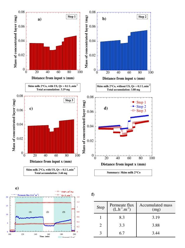
Fig. 7 Matter accumulation of concentrated layer along x axis during filtration of skim milk suspensions (feed:  $2*C_o$ ).  $T = 25\pm1°C$ ,  $TMP = 1.1\times10^5$  Pa. US: 20 kHz, 2 W.cm<sup>-2</sup>. a-d: mass profiles; e: reminder of permeate flux  $J_v$  curve for step 1 to 3; f: table of values for each step at steady state.
