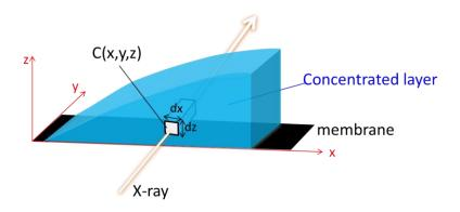
Fig. 4 Schematic of concentrated layer on the membrane surface
