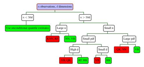
Figure 1: Method recommendation depending on the problem at hand (green: recommended methods, red: methods to avoid). KN: nearest-neighbors, RF: random forests, NN: neural networks, RK: RKHS regression, QK: quantile kriging, VB: variational Bayesian.
