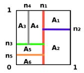
Figure 3: Left: a partitioning tree T. The nodes  $n_i$   $(1 \le i \le 5)$  represent the splitting points, the  $A_i$ 's  $(1 \le i \le 6)$  represent the leaves. Right:  $\mathcal{X} = [0,1]^2$  as partitioned by T. The regression tree prediction is constant on each leaf  $A_i$ .
