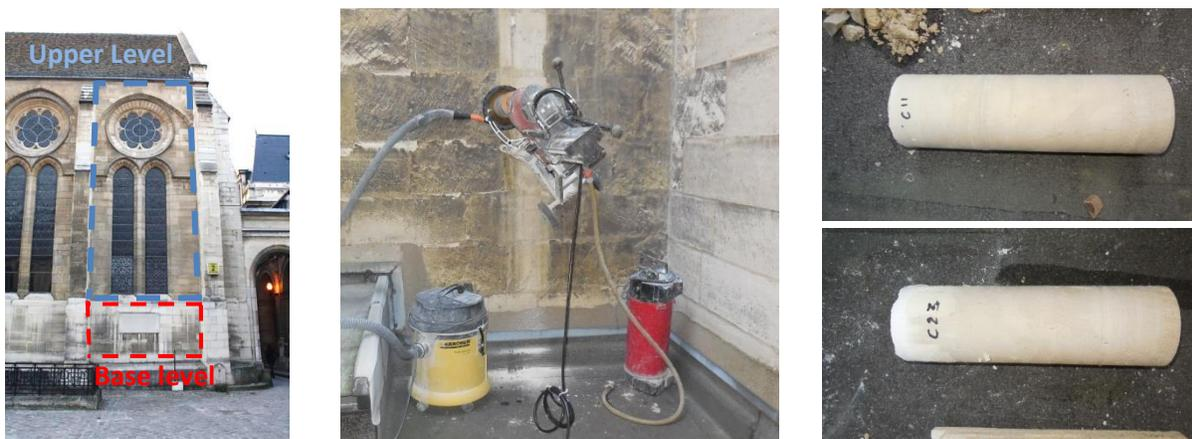
**Fig 2.** Cores drilled out on the monument
