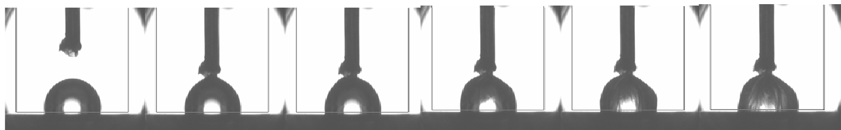
Fig. 2: Snapshots of hydrate growth at 27 bar, 5°C in a CO 2 /pure water system showing film growth from the top to the bottom of the drop. The water drop is hit at its top by the hydrate hanging at the capillary tip (second image from the left), initiating hydrate film growth (from left to right). Drop coverage is obtained within 9 s; then most of the water within the drop remains unconverted.
