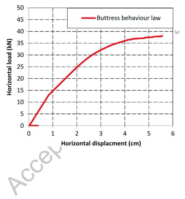
Figure 17. Behaviour law of the buttress, Horizontal load vs Horizontal displacement
