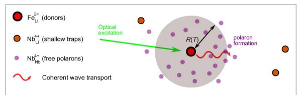
**Figure 6.** Proposed scheme for the interpretation of the photogeneration efficiency. The grey circle represents the volume where the newly formed polarons are likely to be retrapped by the Fe donor. The polarons can form at any distance from the donor center with a given probability distribution (see text).
