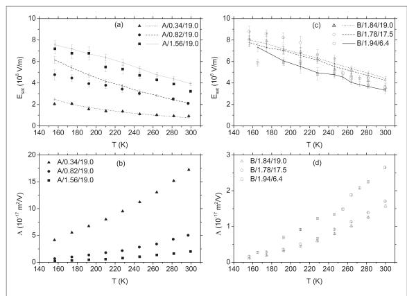
**Figure 2.** (a) Saturation space charge field as a function of temperature for sample series A. Dots: experimental points; Lines: recomputed results taking  $L_{PG}=1.44$  Å and  $\Lambda_0=1.69\times10^{-17}$  m<sup>2</sup>/V (see text for details). (b) Simulated Λ for sample series A. (c) Same as (a) for sample series B. (d) recomputed Λ for sample series B.
