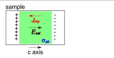
**Figure 1.** Scheme of the experimental geometry: a Fe:LN sample is illuminated with a uniform strip of light. Inside the illuminated volume a current density  $j_{PG}$  and a conductivity  $\sigma_{PC}$  are established. The charge accumulation at the boundaries of the illuminated area give rise to an electric field  $E_{sat}$  that in stationary conditions counterbalances the photogalvanic current.
