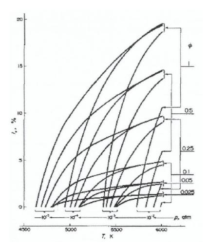
Fig. 2. Percentage of deionization vs de parameters p, T and  $\phi = m_{H,O}/m_{N_2}$ .
