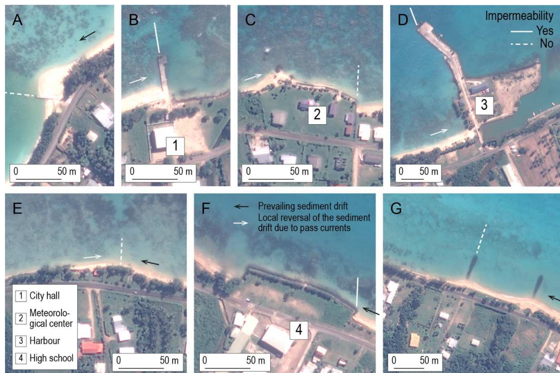
Fig. 5. The boundaries of the eight sub-cells considered in this study and their impermeability. A) Boundary between sub-cell 1 and sub-cell 2; B) Boundary between sub-cell 2 and sub-cell 3; C) Boundary between sub-cell 3 and sub-cell 4; D) Boundary between sub-cell 4 and sub-cell 5; E) Boundary between sub-cell 5 and sub-cell 6; F) Boundary between sub-cell 6 and sub-cell 7; G) Boundary between sub-cell 7 and sub-cell 8. Longshore sediment drift and landmarks shown in Fig. 2B are also indicated. Imagery source: Pléiades satellite imagery (©CNES_2014, Airbus DS Distribution, all rights reserved).
