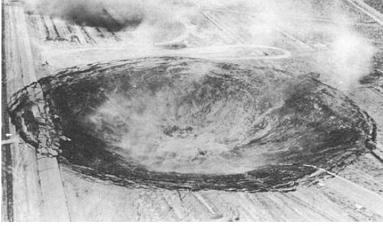
Figure 15: Numerous examples of subsidence craters created by underground nuclear explosions can be found for instance at Nevada test site in the USA. Although this one is in tuf, hard rocks such as granite can also produce a similar, counter-intuitive phenomenon.
