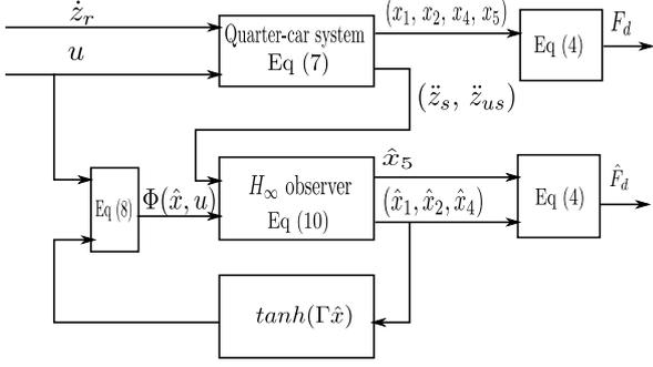
Fig. 3. Block diagram of the  $\mathcal{H}_\infty$  damper force observer
