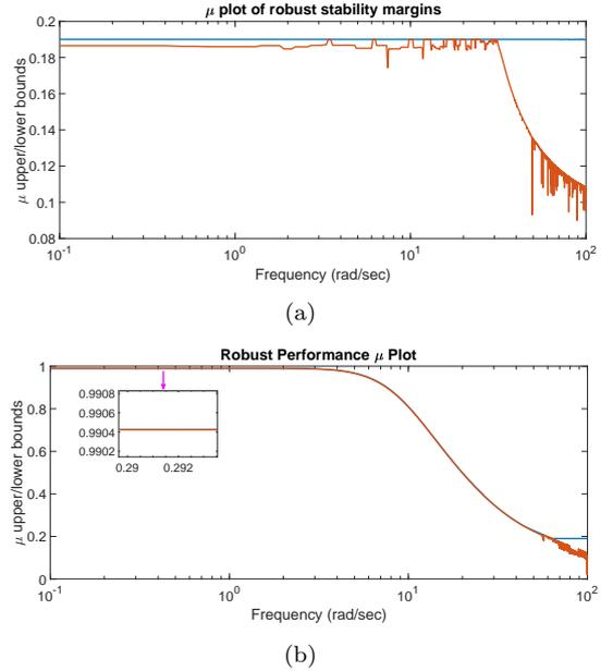
Fig. 9. (a) Robust stability analysis, (b) Robust performance analysis
