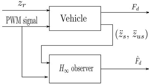
Fig. 11. Block diagram for implementation of the  $\mathcal{H}_\infty$  damper force observer
