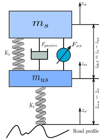
Fig. 1. 1/4 car model with semi-active suspension
