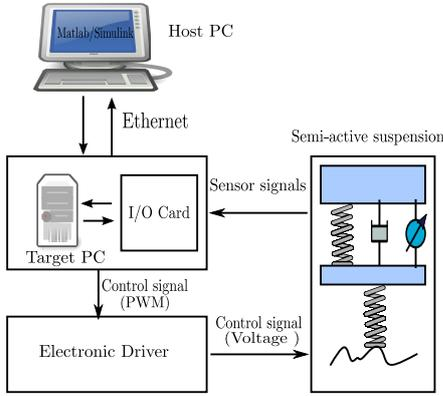
Fig. 2. Schematic diagram of testbed of semi-active suspension system
