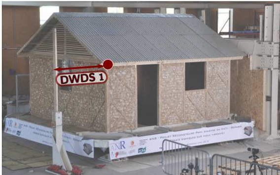
Figure 8: Experimental specimen tested under dynamic loading and its modeling: (a) House subjected to dynamic loading -- Top shear wall displacement recorded via a Draw Wire Displacement Sensor (DWDS) (b) Simplified FE model of the house using macro-element assembly
