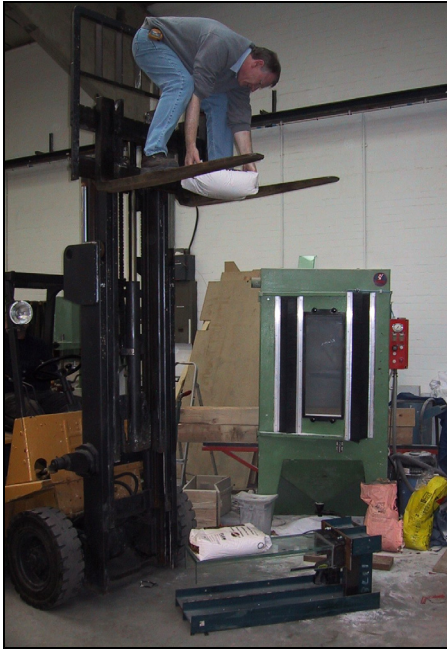
Fig. 8: Drop test with a 25kg weight landing on the End of the tread, \Delta H \sim 4m , no failure
