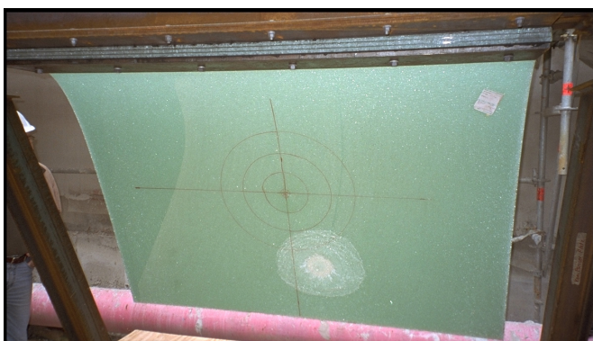
Fig. 10: failure of the lowest pane TG at a drop height 3.0 m
