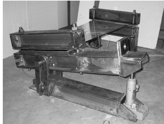
Fig 2: Test set-up for torsional tests
