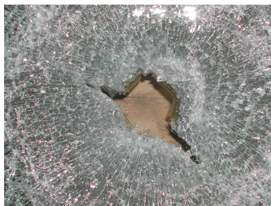
Fig 22 Fractured fabric around the glass hole
