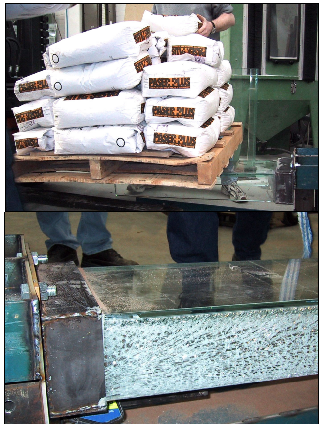
Fig. 6: Testing set- up with sand- bag loading for P 1 (top); primary crack at centre of inner laminate of flange (bottom)
