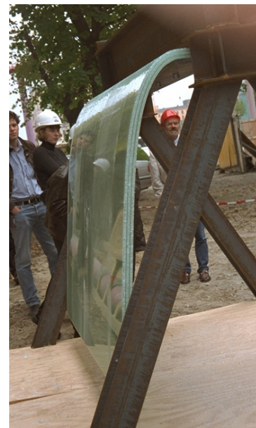
Fig. 12: Broken TG forced into vertical position
