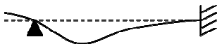
Fig 15: One side hinged supported and the other side restrained supported beam with a projecting end
