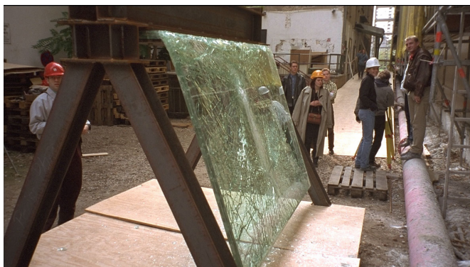
Fig. 15: Test HSG pressed into vertical position
