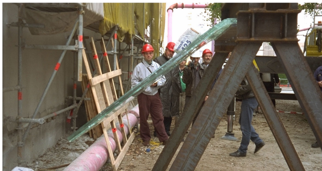
Fig. 14: Test HSG (failure of all panes)
