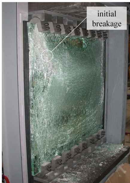
Fig 23: Buckled glass plate.
