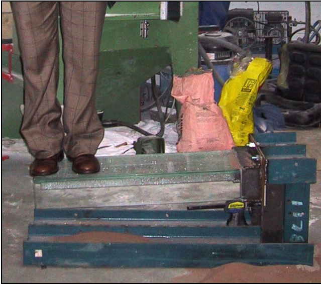
Fig. 11: Sufficient post- failure security observed
