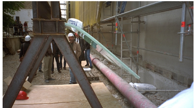
Fig. 11 Failure of all panes TG after an impact from 10 m
