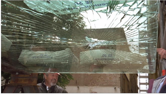
Fig. 13: Test HSG (failure uppermost pane)
