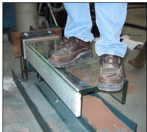
Fig. 10: Both panels of one flange broken, tread still carries one person
