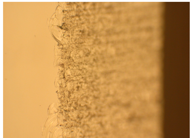
Fig 5: Abrided edge of the annealed float glass
