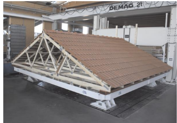
Figure 6: Roof setup for dynamic test
