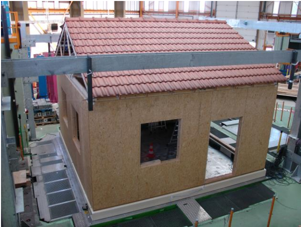
Figure 10: Overview of the house on the shaking table
