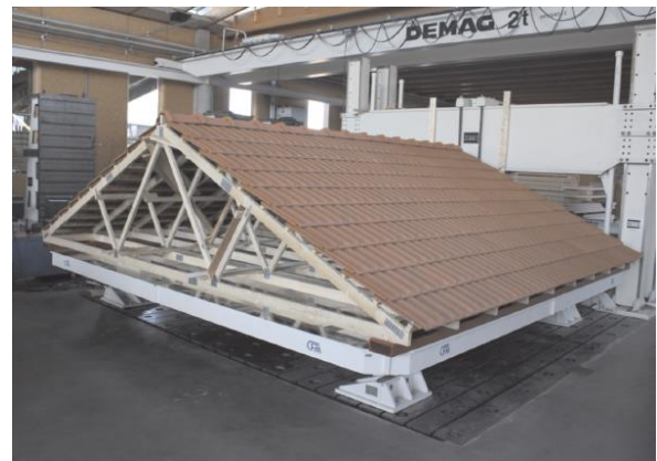
Figure 6: Roof setup for dynamic test
