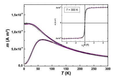
**Fig. 3** (color online) Magnetic characterization of the 4.7 nm sample. Shown are the experimental ZFC/FC curves at 5 mT and the m(H,T) magnetization curve at T=300 K (points) together with the fits (solid lines).
