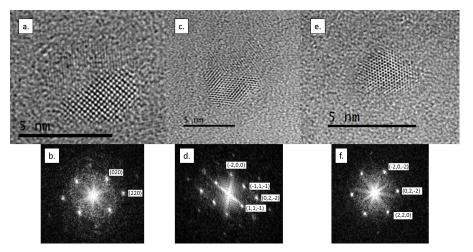
**Fig. 2** HR-TEM images and the respective Fourier transform patterns of cobalt nanoparticles embedded in amorphous carbon. The particle diameters (mean of the two half axes) and orientations are, respectively: a, b: 4.6 nm [0,0,1]; c, d: 5.0 nm [0,1,1] and e, f: 2.8 nm [-1,1,1].
