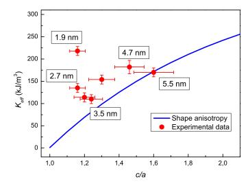
Fig. 5 (color online) Experimental variations of the magnetic anisotropy constant  $K_{eff}$  as a function of the aspect ratio c/a. The horizontal bars for the experimental data correspond to the dispersions of the aspect ratio as estimated from TEM. The blue line shows the calculated shape anisotropy constants.
