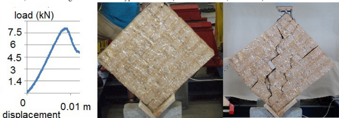
Fig 2: a) experimental vertical stress/strain curve b) Shear test by 45° compression of the adobe assembly . c) End of the test
