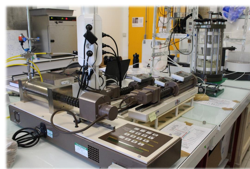
Unconventional triaxial system
