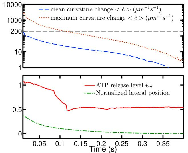
FIGURE 13 The upper panel shows the history of mean and maximal curvature change during the migration process at  $(Ca, Cn) = (50, 0.3)$ . The horizontal gray dashed line corresponds to the value of the critical curvature change  $\dot{c}_c = 200 \mu\text{m}^{-1}\text{s}^{-1}$ ; the lower panel shows the ATP release level and normalized lateral position history at  $(Ca, Cn) = (50, 0.3)$ . To view this figure in color, go online.
