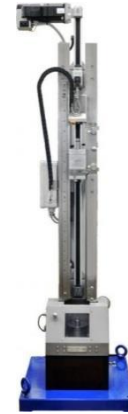
Figure 6. BAM fall hammer (OZM Research) used for impact tests carried out on our monopropellant prototypes
