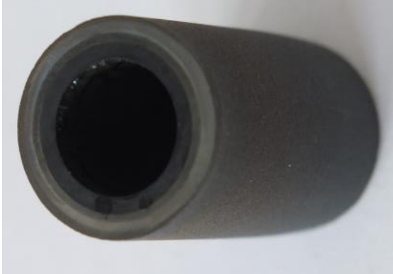
Figure 12. Example of UHTM sample obtained by additive manufacturing in the frame of this project
