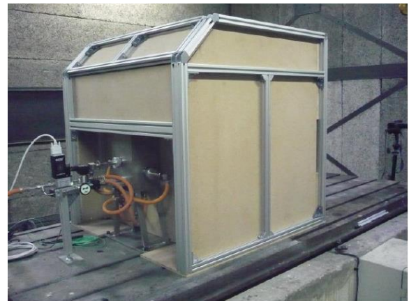
Figure 6. BAM fall hammer (OZM Research) used for impact tests carried out on our monopropellant prototypes
