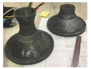
Figure 35: Design description of the different parts of the CC-SiC nozzle © Nammo
