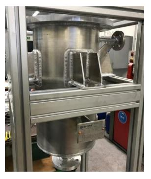
Figure 28: PROPULSE 980 aluminium reactor for HTP crystallization production plant. © Evonik
