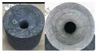
Figure 17: Pre- & Post-firing inspection of a CC-SiC nozzle breadboard © Nammo
