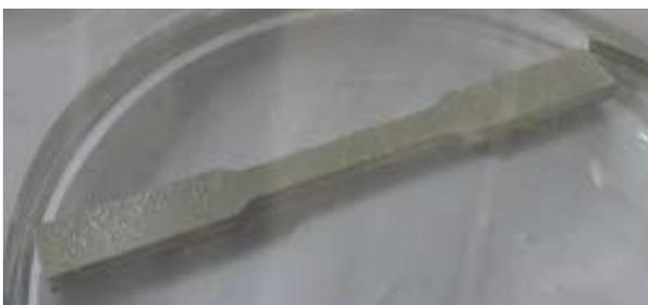
Figure 20: Material compatibility tests with HTP © Airbus DS GmbH
