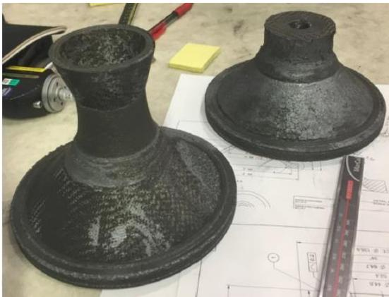
Figure 35: Design description of the different parts of the CC-SiC nozzle © Nammo
