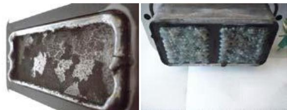
Figure 15: Post-test inspection of several concepts of isochoric combustion chambers © Onera
