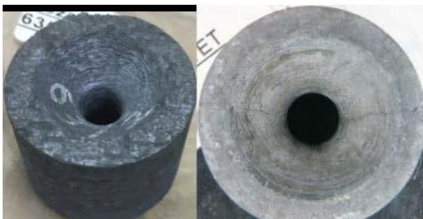
Figure 17: Pre- & Post-firing inspection of a CC-SiC nozzle breadboard © Nammo
