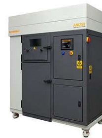
Figure 11. Renishaw AM250 Printer Used for Manufacturing the Injector Ducts.
