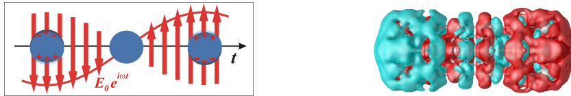
Figure 2 – Left panel: schematic of the classical picture of the SPR as a density oscillation. Right panel: Snapshot of the density dynamics showing the longitudinal charge oscillation in a 37-atom Ag nanorod (cf., Ref. [4]).
