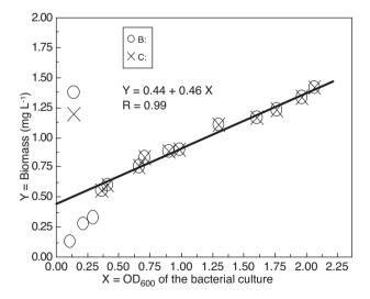
Calibration of the spectrophotometer for a reading in mass dries; (0) Distribution of the mass dries vs. OD<sub>600</sub> of the bacterial culture; (x) Correlation curve of the experimental points located in the field of the validity of the Beer-Lambert law.
