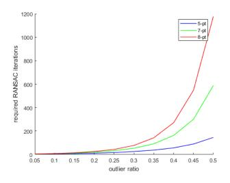
Fig. 4. Required RANSAC iterations vs outlier ratio.
