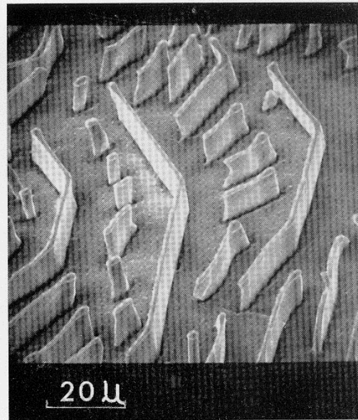
Fig. 8. — Fibres et rubans. V = 1 cm/h, G = 70^\circ /cm.
