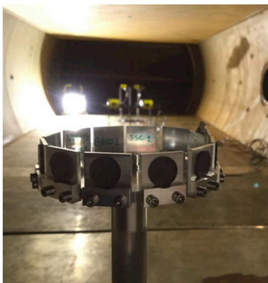
Fig. 4. Laser targets on the specifically designed sample wheel.
