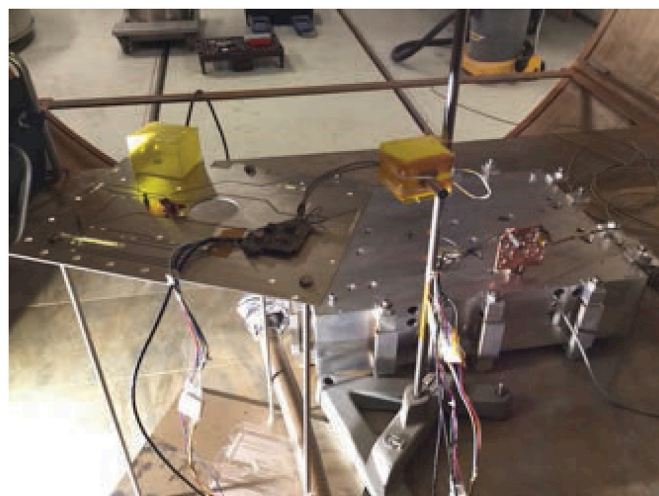
Fig. 5. Photo of the two microphones installed on the cooling plate using a copper support. Another microphone, also seen in the photo, was placed on a mechanical support as close to the cooling plate as possible (not thermally coupled). The electronics of this microphone were left attached to the PCB support used during the first test configuration.
