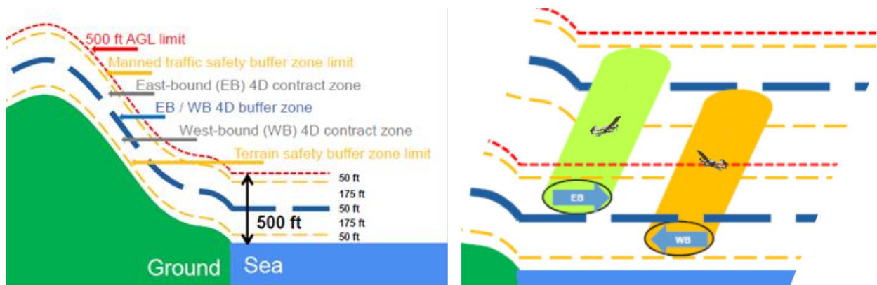
Figure 1: Semi-circular rule for RPAS VLL operations and perspective view of the RPAS traffic.
