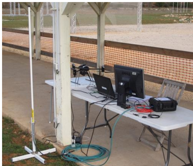
Figure 5: The ground LLRTIM station with the high gain antenna used in the demonstration of RPAS remote identification.
