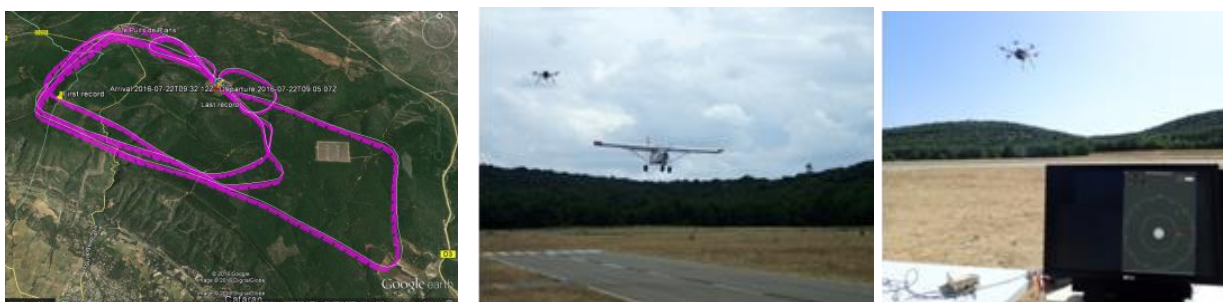
Figure 4: Illustration of first flight tests, showing the flown intruder trajectories, a conflict situation between the RPA and the intruder, and the LLRTM ground segment with the display intended for use by the remote pilot.
