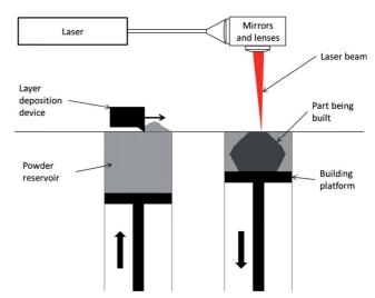
Fig. 1 Schematics of the selective laser sintering/melting process
