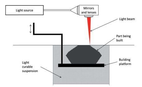
exposure are two adjustable parameters allowing the control of the energy sent to the resin.
