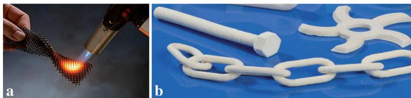
**Fig. 3** Examples of ceramic parts manufactured by stereolithography. **a** SiC ceramic mesh manufactured by HRL (Courtesy of HRL Laboratories, Photo by Dan Little) [40] **b** Alumina parts (Courtesy of CTTC)
