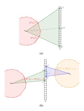
Figure 6: View of the 2-flat  $\mathcal{P}$ : (a) Binary search initialization to compute the wedge  $(a, \mathcal{F}^a(e))$ . (b) After completion of two binary searches, both wedges  $(a, f_k = \mathcal{F}^a(e))$  and  $(a, f_l = \mathcal{F}^b(e))$  are known.
