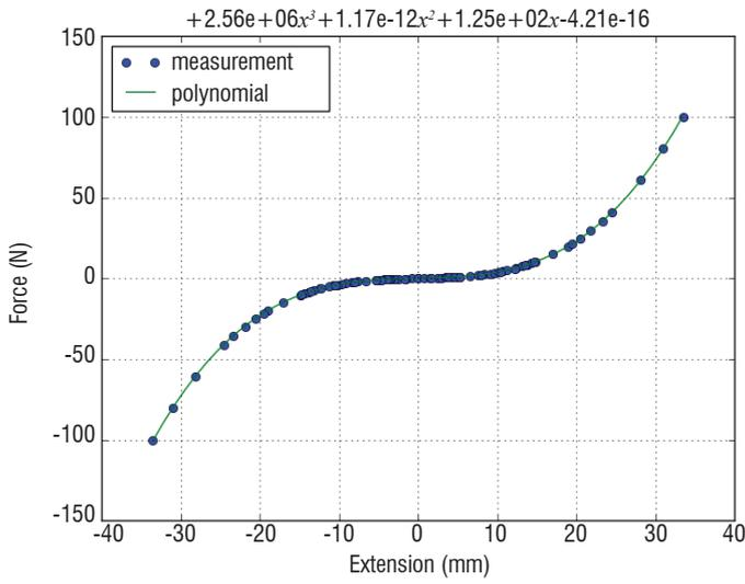
Figure 6 – Static force identified with weights
