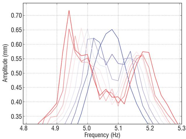
Figure 12 – Zoom on the primary structure spectra
