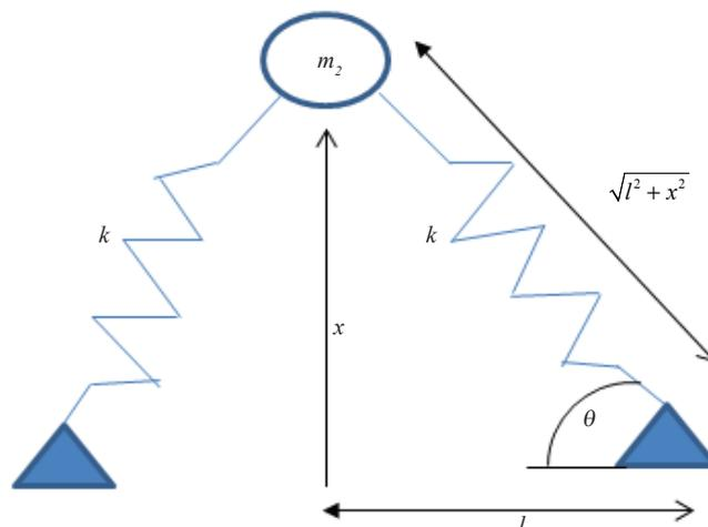
Figure 5 – Simplified movement model of the NES
