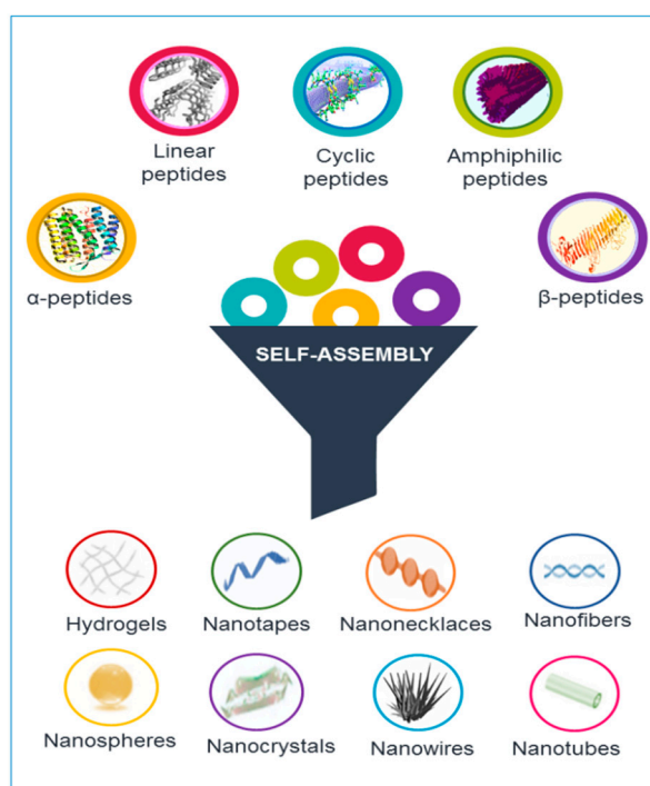
Figure 1. Different classes of peptides can be arranged in supramolecular structures handling the self-assembling phenomena. Various morphologies can be generated according to the rational design of the primary sequence.
